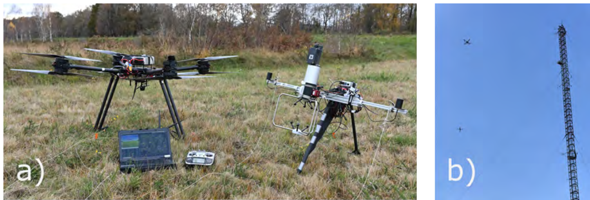
Figure 2: a) Overview of the SAMURAI-S system featuring a Foxtech D130 UAV with a custom-made payload that includes an RM Young 81000 sonic anemometer. b) The system performing a validation flight close to a 60m mast.
