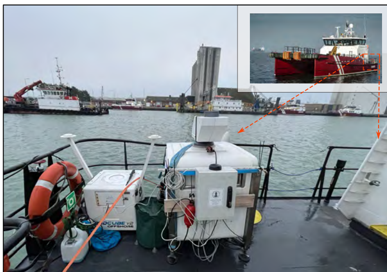
Figure 3: Lollex experiment: Temporary installation of lidars onboard the CTV. The WindCube V2 lidar wind profiler (left) and WindCube 100S scanning wind lidar (right) were installed on the stern side in the back of the vessel.
