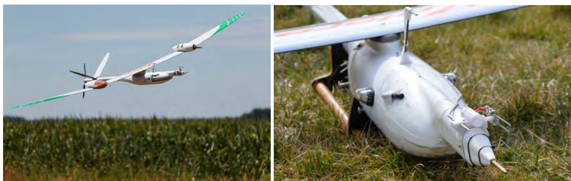
Figure 1: MASC with its sensorhood mounted on during flight campaign in Lindenberg, Germany. Source: B. Lammel
