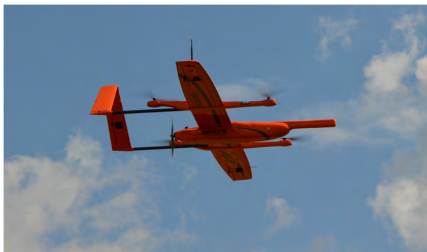
Figure 1: Multipurpose Airborne Sensor Carrier MASC-V during vertical landing. The FHP is mounted at the tip of the nose boom, far in front of fuselage, wings, and rotors.
